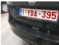
Bumper R, Scratch(es), Repair and paint (complete)
