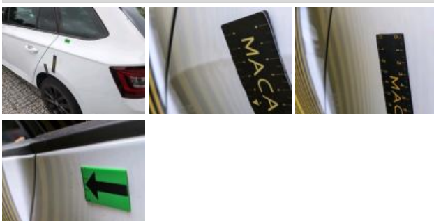
Wing RL, Dent(s), Paintless dent repair
