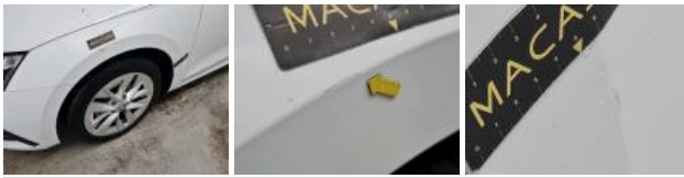
Bumper F, Scratch(es), Repair and paint (complete)
