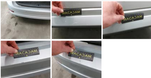
Tailgate / Boot, Dent(s) and scratch(es), Acceptable
