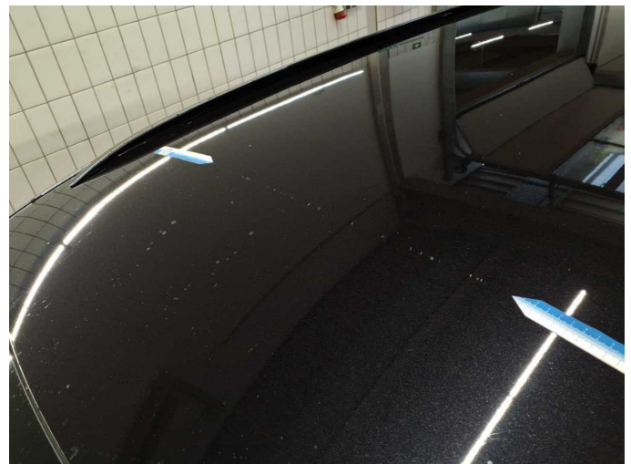
Damage 11: Roof: Roof - Scratch(es) - Paint
