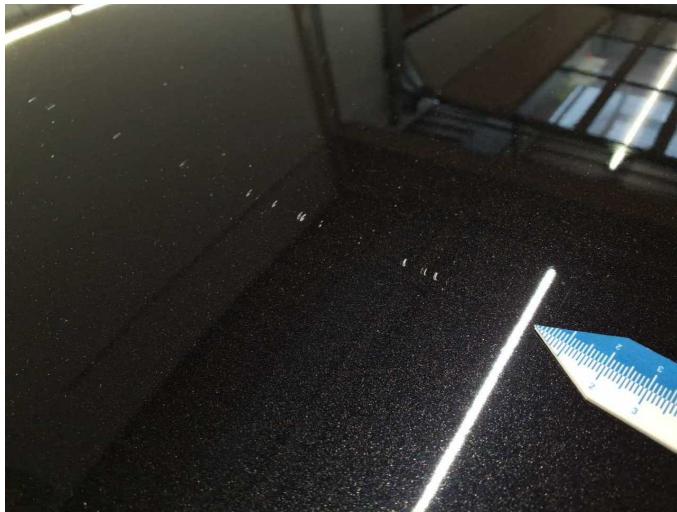
Damage 11: Roof: Roof - Scratch(es) - Paint
