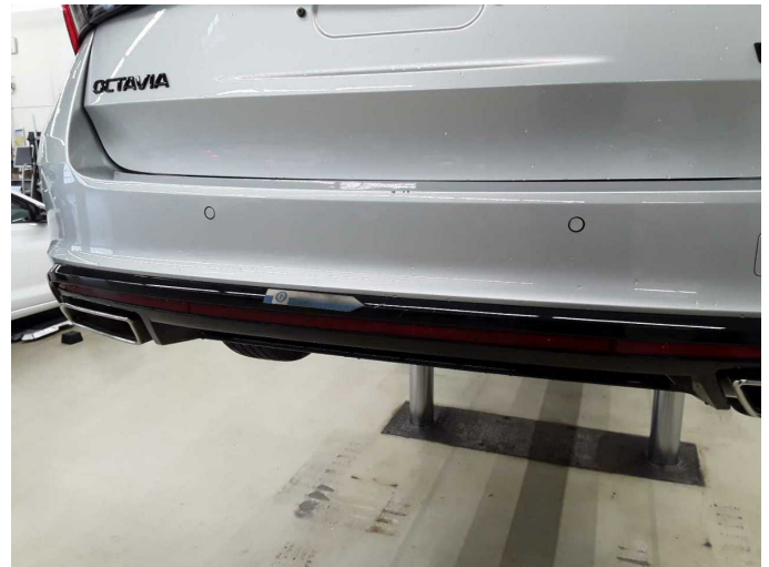
Damage 7: Rear bumper: Rear bumper (Incl. Schwarzer Zierleiste) - Damaged - Smart repair
