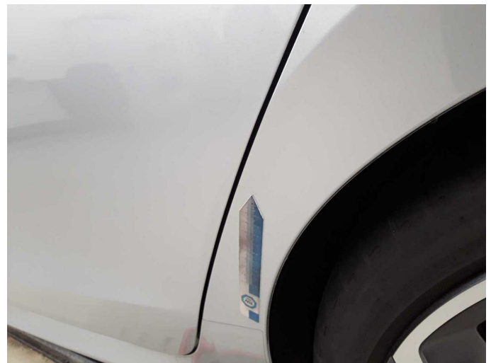
Damage 2: Side panel - rear left side: Wheel arch - dent(s) - Smooth repair work
