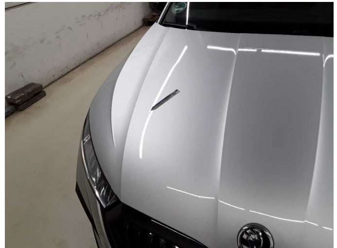
Damage 1: Bonnet: Bonnet - dent(s) - Smooth repair work
