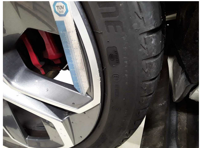
Damage 5: Wheel / tyres: Alloy rim - rear right side - Damaged - Loss in value
