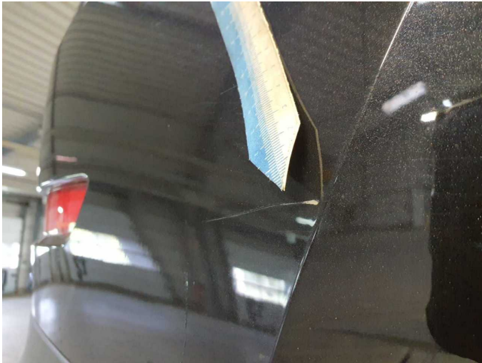
Damage 4: Rear bumper: Rear bumper - Scratched - Paint
