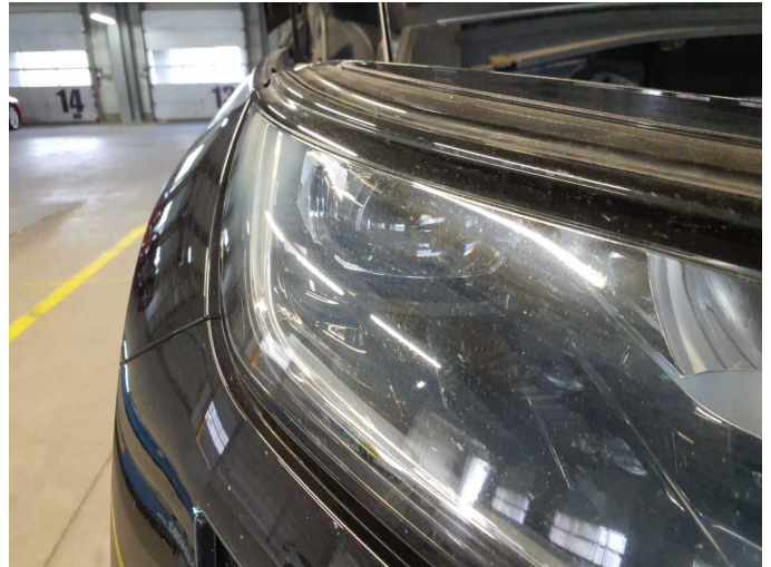
Damage 10: Headlight: Headlight - right side (Scheinwerfer blind/Milchig) - Damaged - Replace
