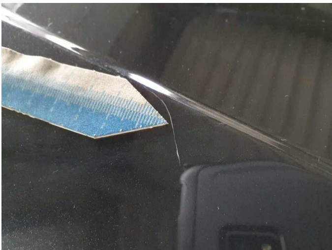
Damage 7: Bonnet: Bonnet (Kratzer) - Stone chips - Paint
