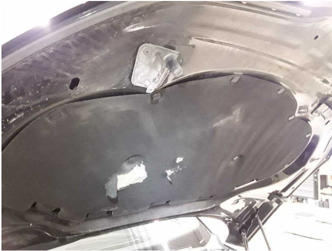
Damage 3: Bonnet: Insulation lining - Broken / torn - Replace
