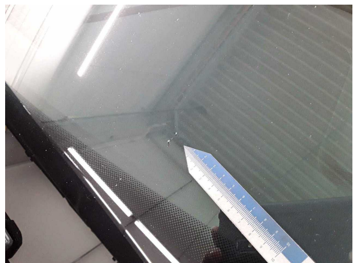
Damage 5: Vehicle glazing: Windscreen - Stone chips - Replace
