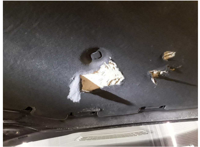
Damage 3: Bonnet: Insulation lining - Broken / torn - Replace
