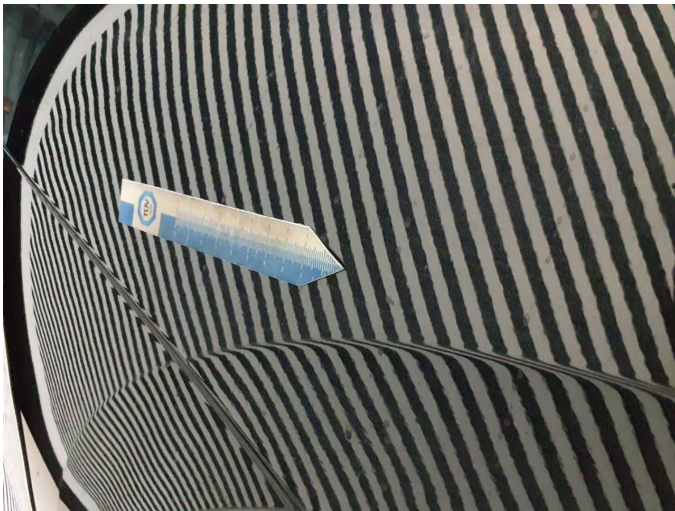
Damage 5: Side panel - rear right side: Side panel - Scratched - Smart repair
