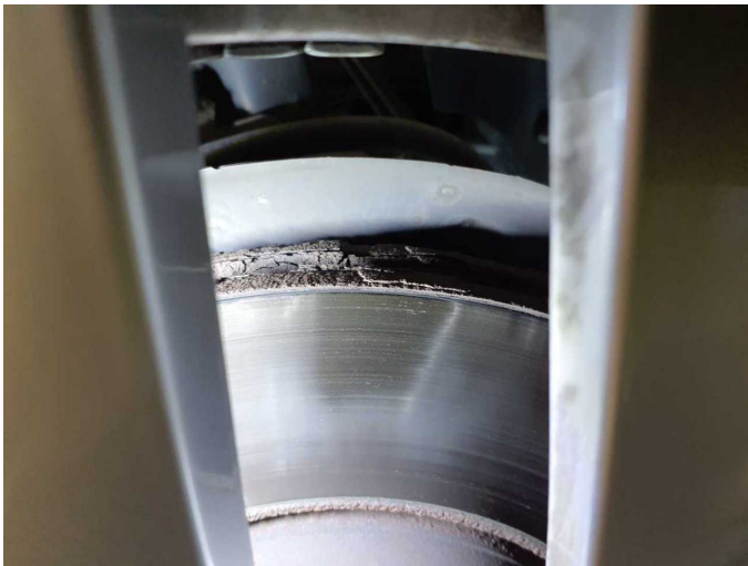
Damage 14: Braking system: Brake discs - front (Tragbild mangelhaft, Rostrand) - Corrosion - Replace
