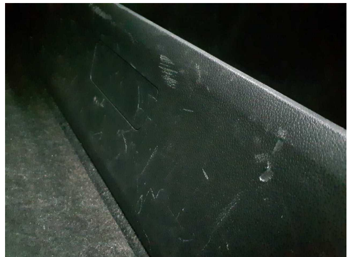
Damage 11: Trim / covers: Cargo area - lining - right side - Scratched - Replace
