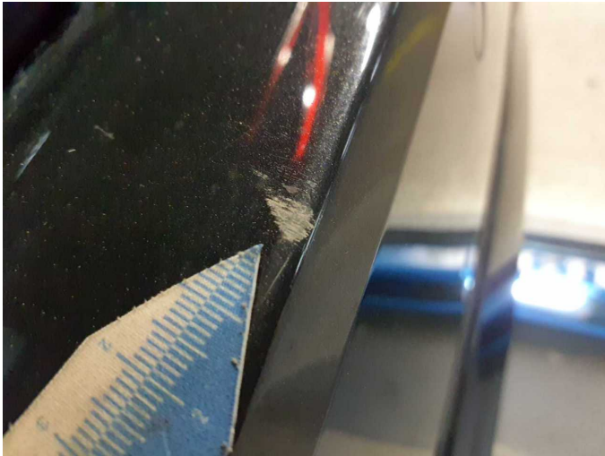
Damage 13: Rear bumper: Rear bumper - Scratched - Paint
