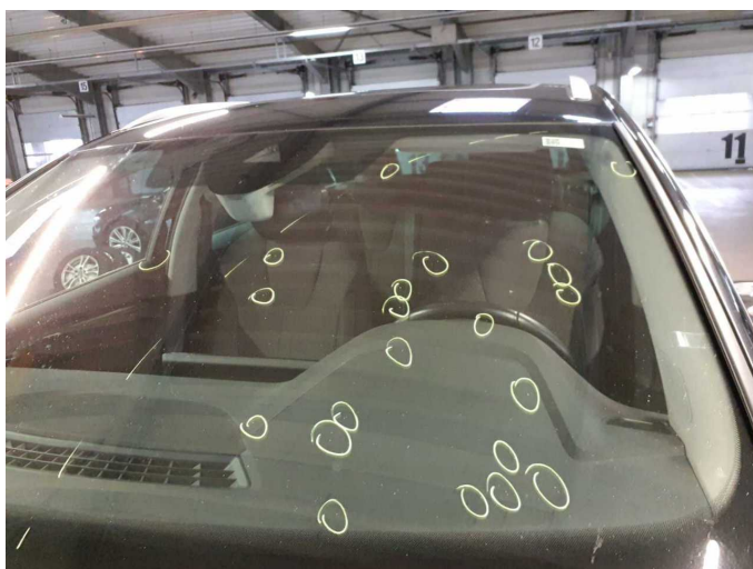
Damage 17: Vehicle glazing: Windscreen (Sandstrahleffekt, Blendwirkung) - Stone chips - repair according to calculation
