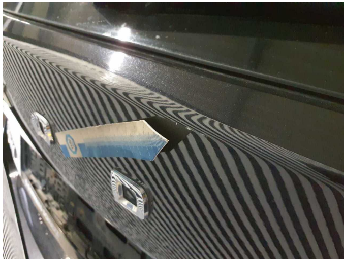
Damage 7: Boot lid / rear door: Boot lid - Scratched - Smart repair
