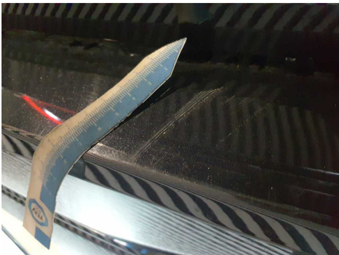
Damage 13: Rear bumper: Rear bumper - Scratched - Paint
