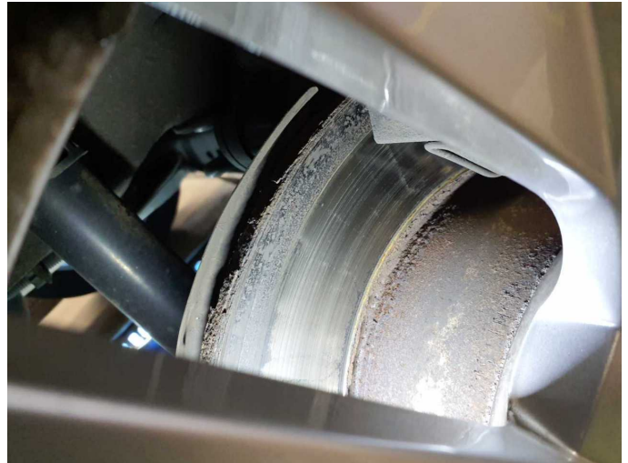
Damage 12: Braking system: Brake discs - rear (Tragbild mangelhaft, Rostrand) - Corrosion - Replace
