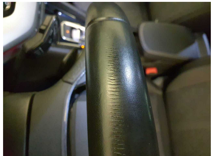
Damage 6: Steering system: Steering wheel - Scratched - Smart repair
