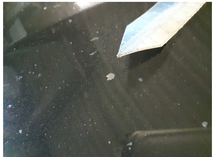
Damage 16: Bonnet: Bonnet (Korrosion) - Stone chips - Repair and paint
