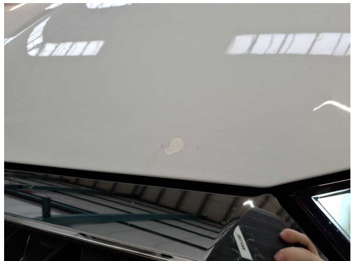
Damage 10: Bonnet: Bonnet - Unprofessionally repaired - Paint
