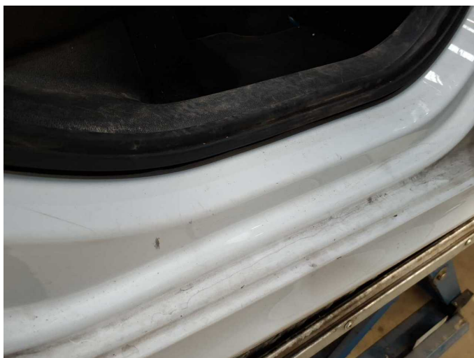
Damage 3: Side panel - rear right side: Sill - Scratch(es) - Cover / polish
