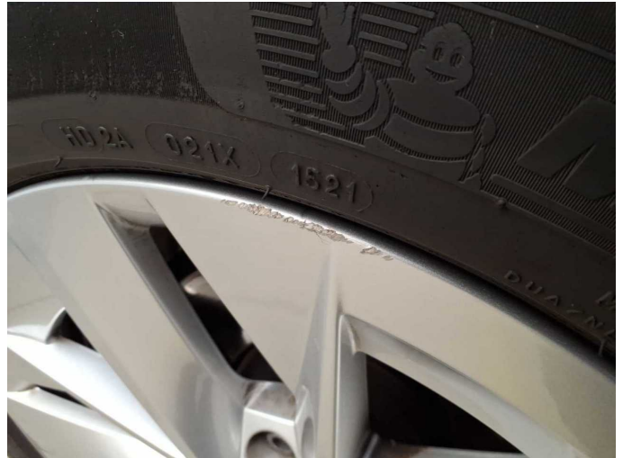
Damage 6: Wheel / tyres: Alloy rim - front left side - Scratch(es) - Loss in value
