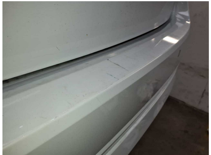
Damage 9: Rear bumper: Rear bumper - Scratch(es) - Paint
