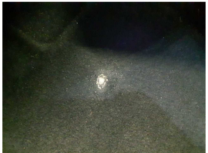
Damage 5: Trim / covers: Carpet - front left side - Holes - Loss in value
