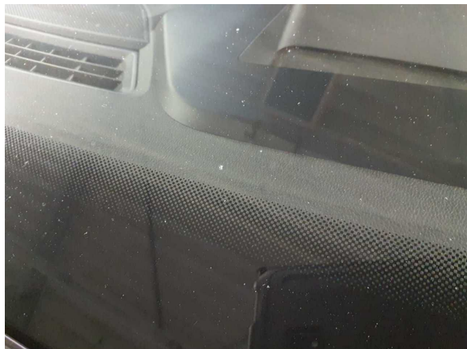
Damage 6: Vehicle glazing: Windscreen with lane departure assistant - Stone chips - Paint
