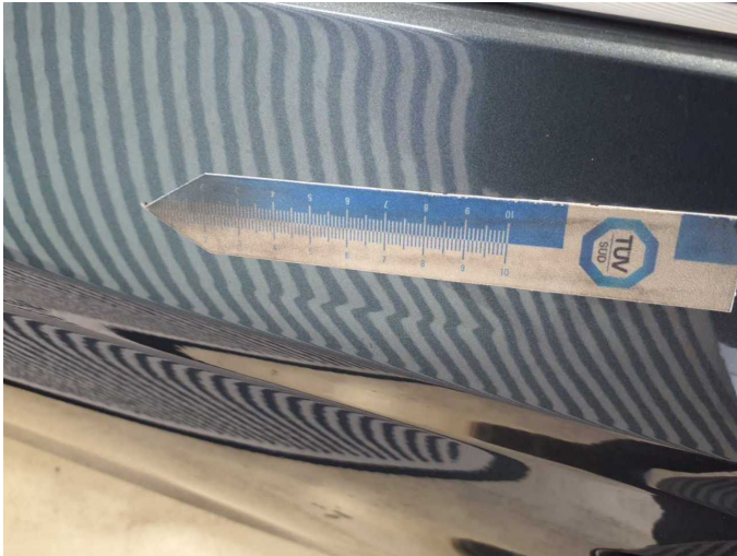
Damage 5: Door - rear left side: Door - Deformed - Repair and paint
