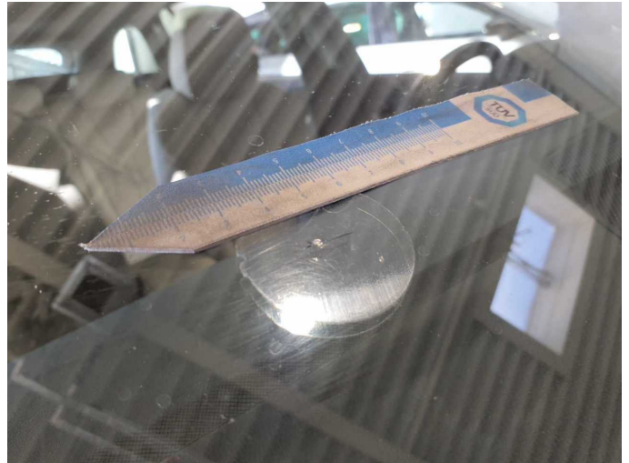
Damage 6: Vehicle glazing: Windscreen - Damaged - Replace
