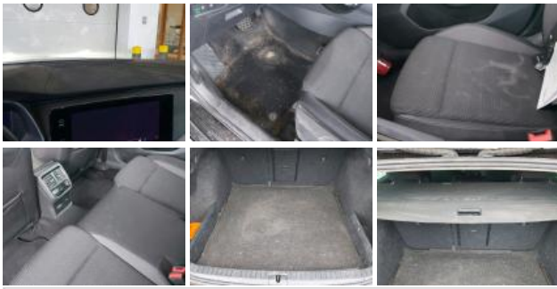
Floor covering FL, Damaged, Replace
