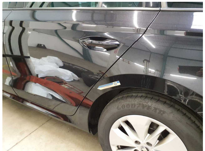
Damage 1: Side panel - rear left side: Side panel - Dent / paintcoat damage - Repair and paint
