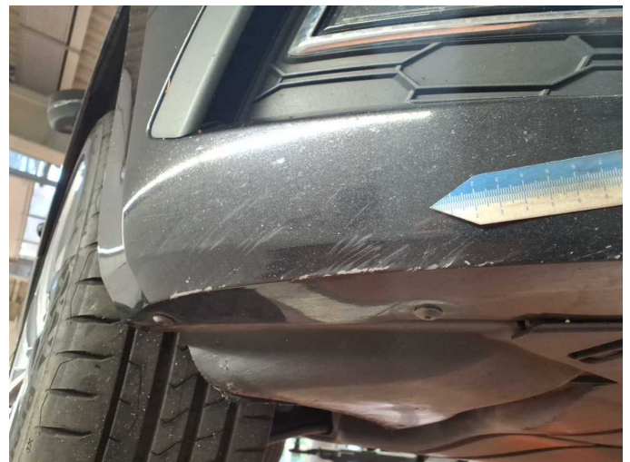
Damage 13: Front bumper: Front bumper - Scratched - Paint
