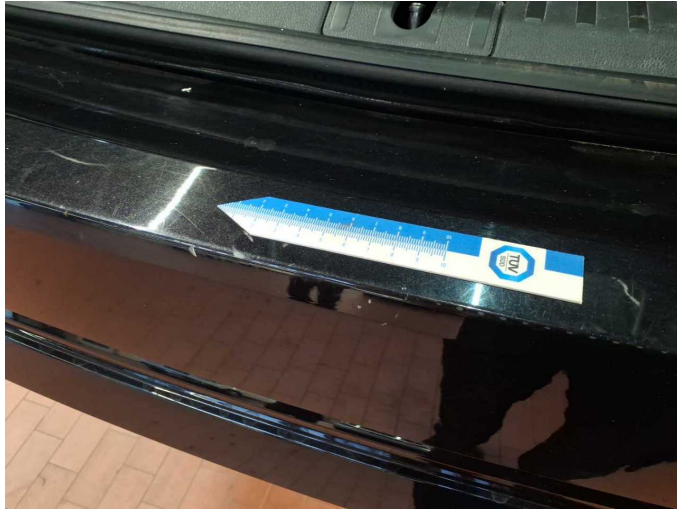
Damage 11: Rear bumper: Rear bumper - Scratched - Paint
