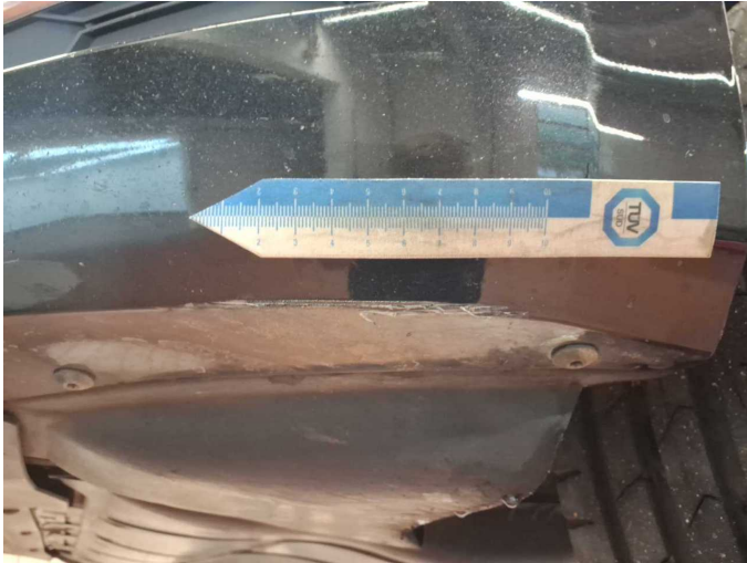
Damage 13: Front bumper: Front bumper - Scratched - Paint
