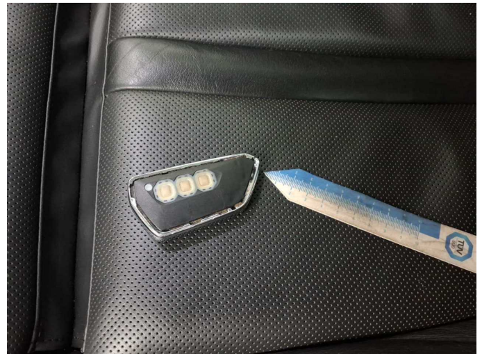
Damage 12: Equipment: Vehicle key with remote control - Broken / torn - Replace
