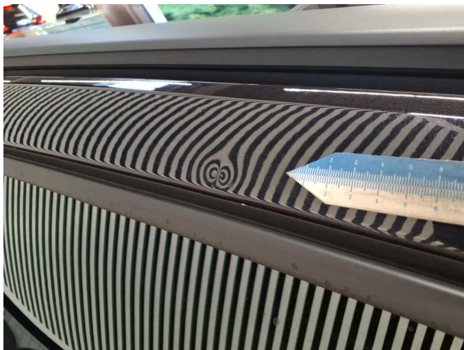
Damage 5: Roof: Roof rail - right side - dent(s) - Smart repair
