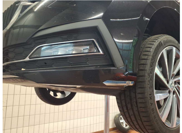
Damage 13: Front bumper: Front bumper - Scratched - Paint
