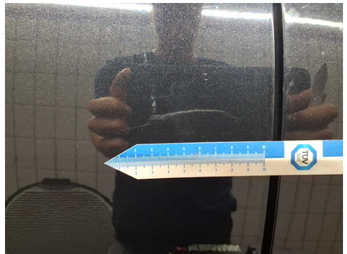
Damage 9: Door - rear right side: Door (an Kante) - Dent / paintcoat damage - Repair and paint
