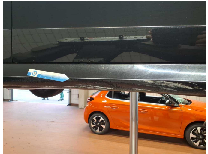
Damage 10: Sill - right side: Sill - Dent / paintcoat damage - Repair and paint
