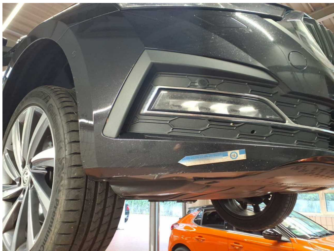
Damage 13: Front bumper: Front bumper - Scratched - Paint
