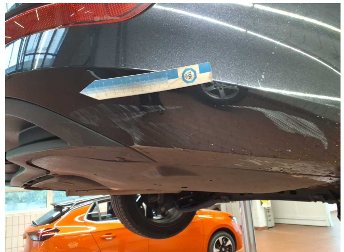
Damage 11: Rear bumper: Rear bumper - Scratched - Paint
