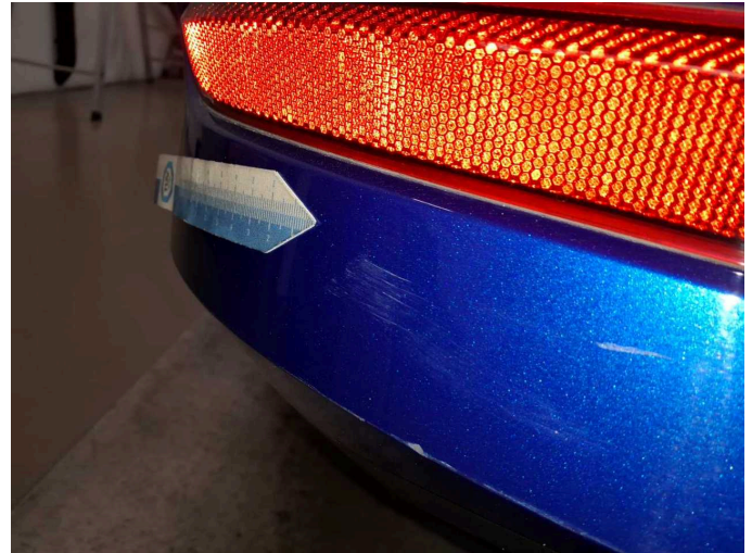
Damage 3: Rear bumper: Rear bumper - Scratch(es) - Paint
