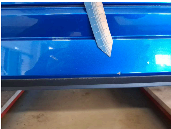
Damage 3: Rear bumper: Rear bumper - Scratch(es) - Paint
