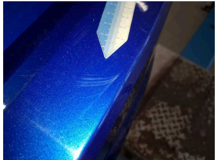
Damage 3: Rear bumper: Rear bumper - Scratch(es) - Paint
