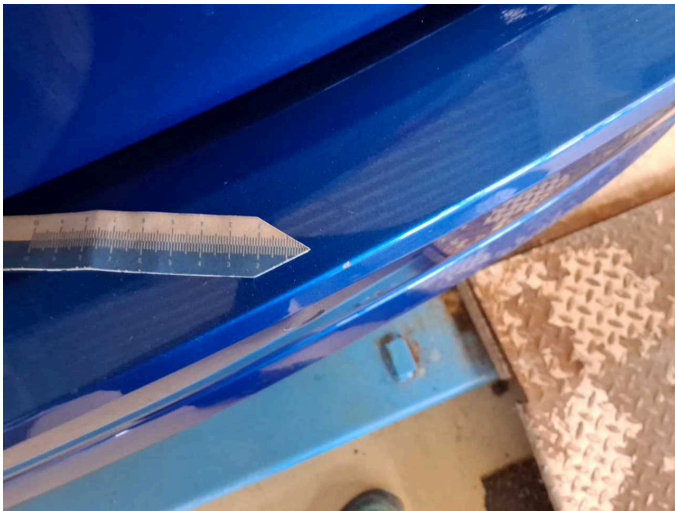
Damage 3: Rear bumper: Rear bumper - Scratch(es) - Paint
