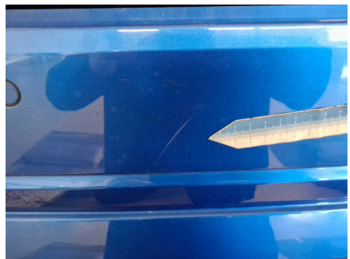
Damage 3: Rear bumper: Rear bumper - Scratch(es) - Paint
