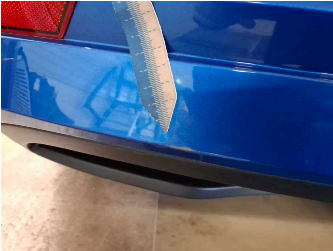
Damage 3: Rear bumper: Rear bumper - Scratch(es) - Paint
