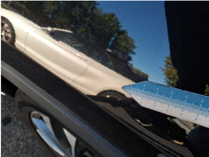
Damage 1: Side panel - rear left side: Side panel - Dent / paintcoat damage - Smart repair
