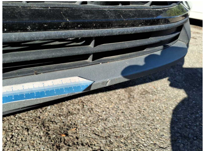
Wear and tear 4: Front bumper: Spoiler - Scratch(es) - No deduction
