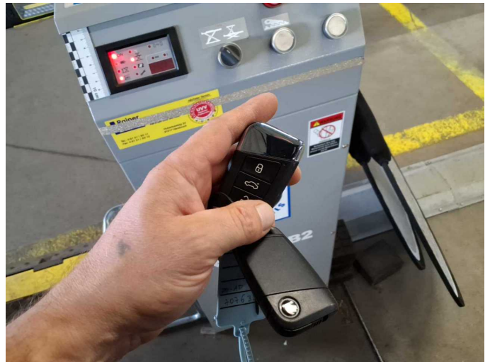
Damage 2: Equipment: Vehicle key (Batterie) - Empty - Replace
