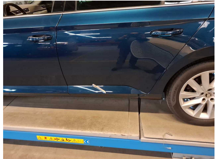
Damage 5: Door - rear left side: Brightware - lower - Scratch(es) - Smart repair
