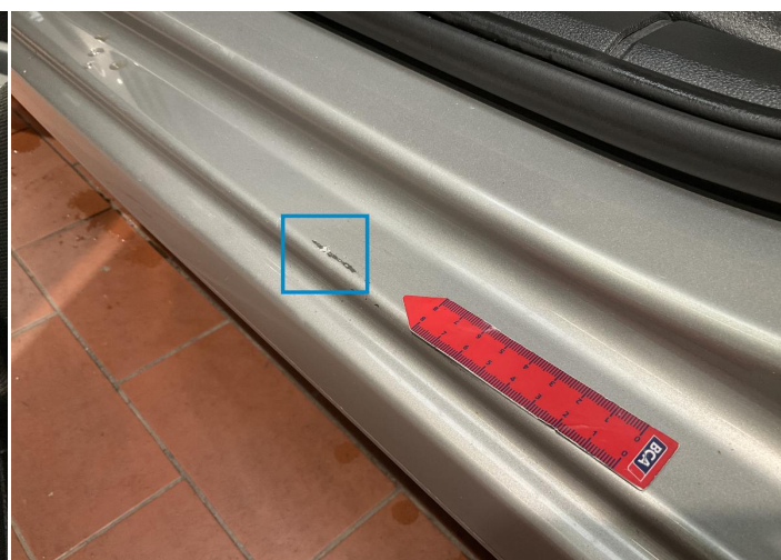
4. B Pillar / Center Left Paint / Scratch / Line -
