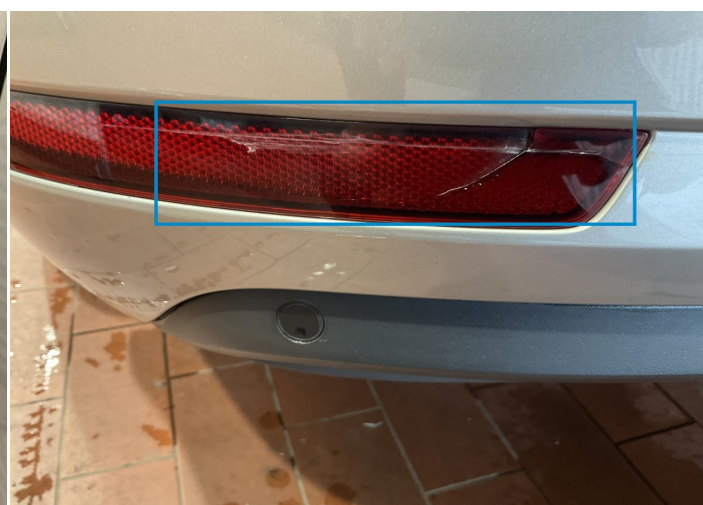
6. Reflector / Back Left Bodywork / Breakage / Crack -
