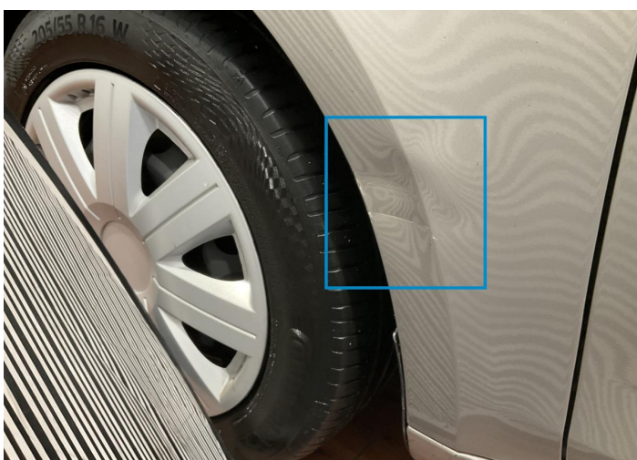
5. Fender / Front Left Bodywork / Dent / Dent -
