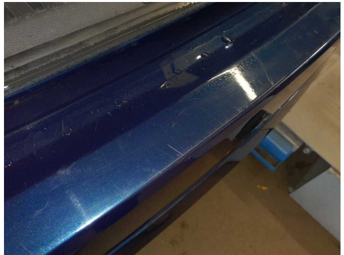
Damage 4: Rear bumper: Bumper - rear centre - Scratch(es) - Smart repair
