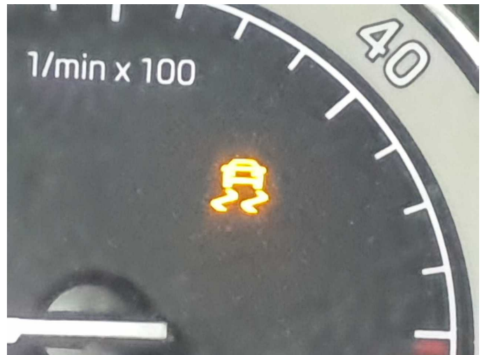
Damage 5: Instrument panel: Indicator light (ESP) - on - Perform diagnosis
