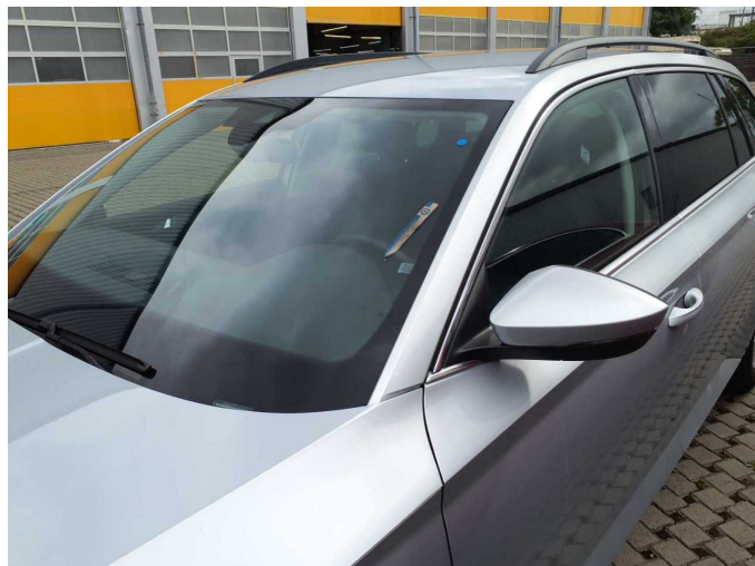
Damage 6: Vehicle glazing: Windscreen - Stone chips - Replace
