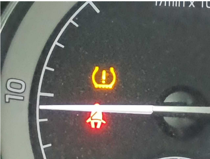
Damage 1: Instrument panel: Indicator light (RDK) - on - Perform diagnosis
