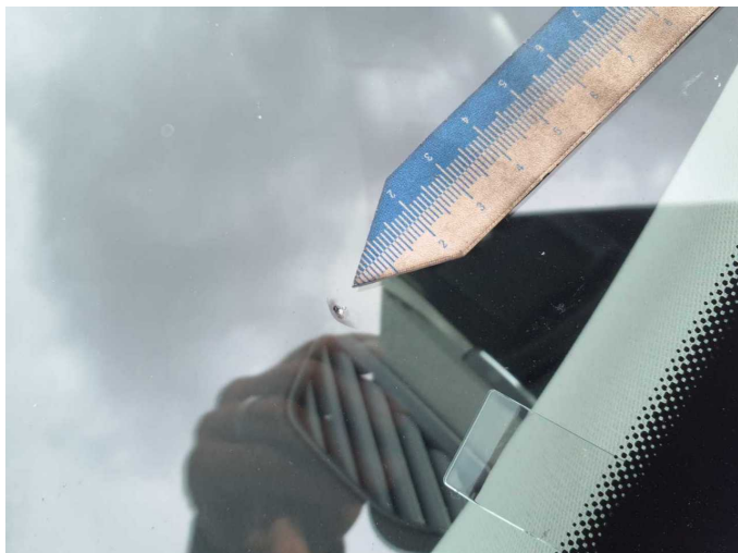
Damage 6: Vehicle glazing: Windscreen - Stone chips - Replace
