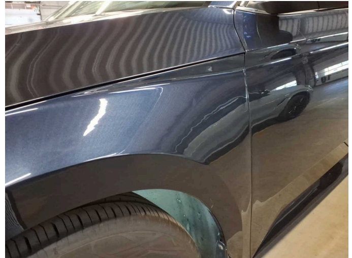
Damage 2: Mudguard - left side: Mudguard - left side (Schleifspuren, wellig) - Unprofessionally repaired - Repair and paint
