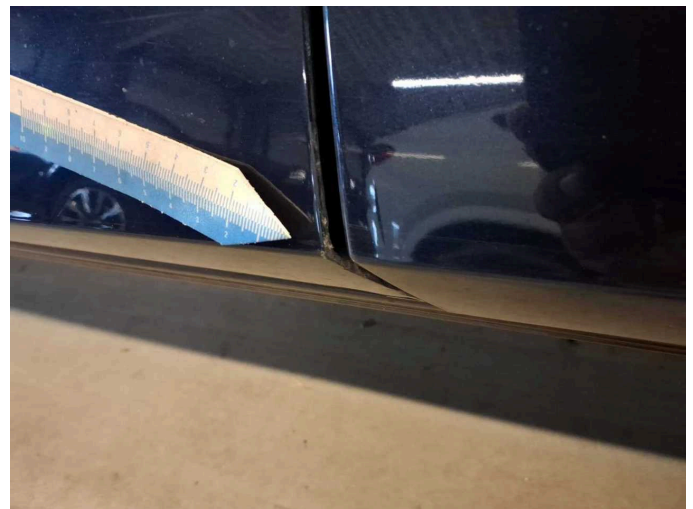
Damage 4: Door - front left side: Door (Wellig) - Unprofessionally repaired - Repair and paint
