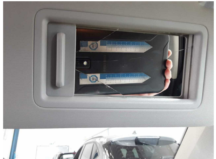
Damage 2: Interior: Sun visor - right side - Damaged - Replace
