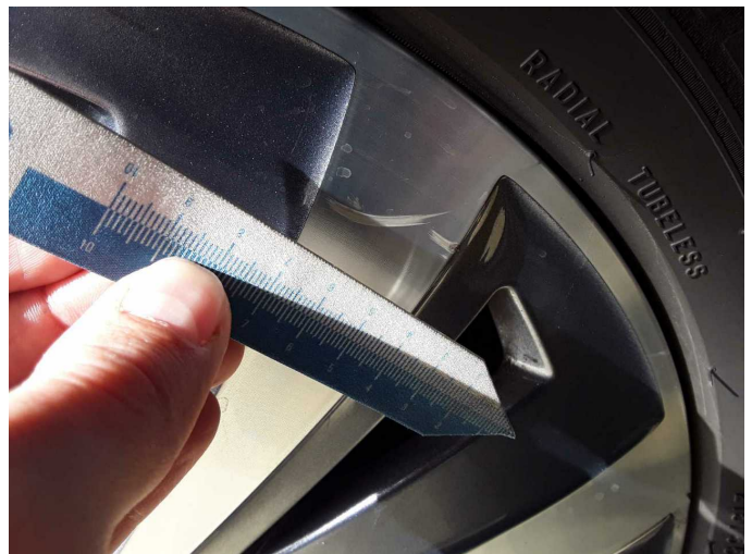
Wear and tear 4: Wheel / tyres: Alloy rim - front right side - Scratch(es) - No deduction
