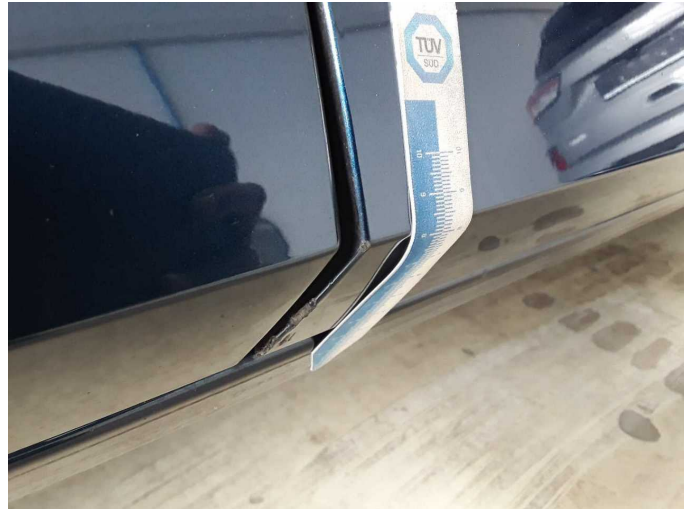
Wear and tear 5: Door - front right side: Brightware - lower - Scratch(es) - No deduction
