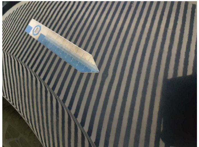
Damage 9: Side panel - rear right side: Side panel - Scratched - Paint
