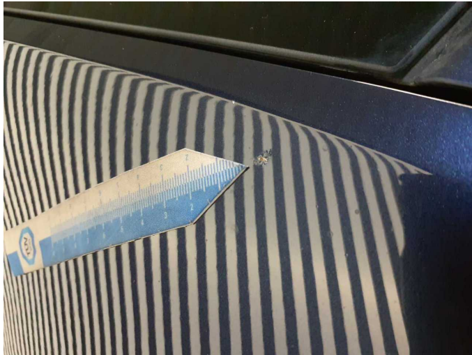
Damage 12: Side panel - rear left side: Side panel - Corrosion - Repair and paint
