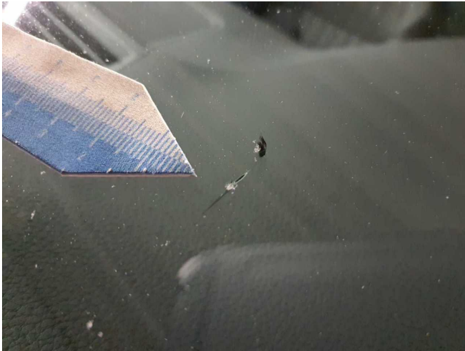
Damage 14: Vehicle glazing: Windscreen (Rissbildung) - Stone chips - repair according to calculation
