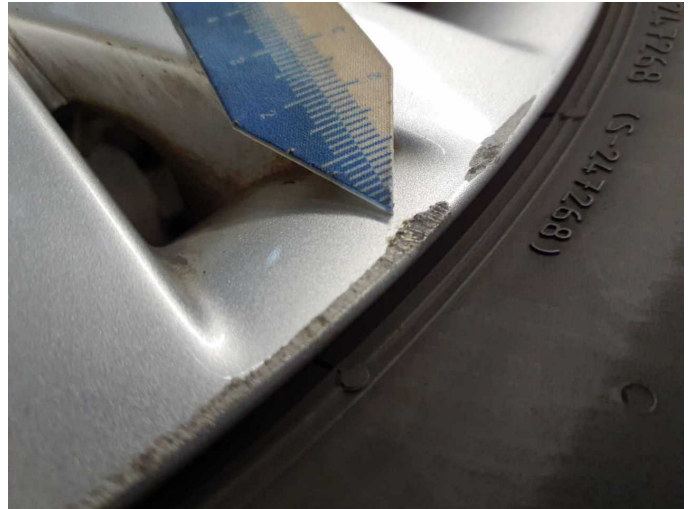
Damage 5: Wheel / tyres: Alloy rim - rear right side (Materialabtrag) - Damaged - Loss in value
