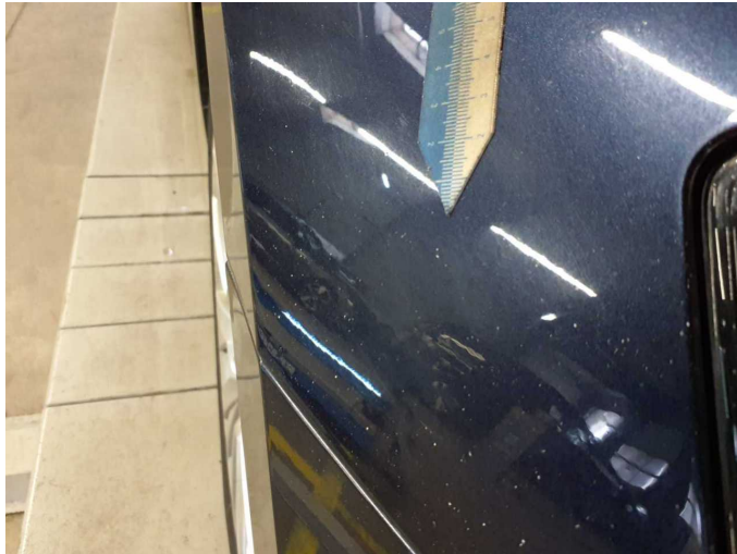
Damage 6: Mudguard - right side: Mudguard - right side (Sandstrahleffekt) - Stone chips - Paint
