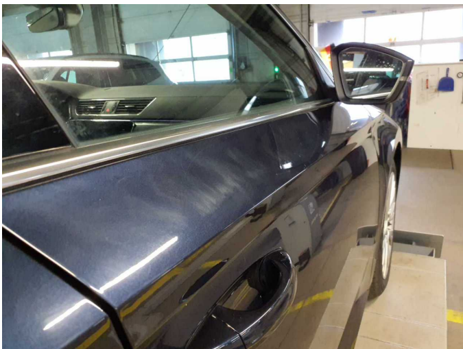
Damage 3: Door - front right side: Door - Scratched - Smart repair
