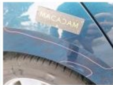
Wing RR, Scratch(es), Repair and paint (complete)
