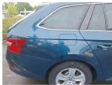
Wing RR, Scratch(es), Repair and paint (complete)
