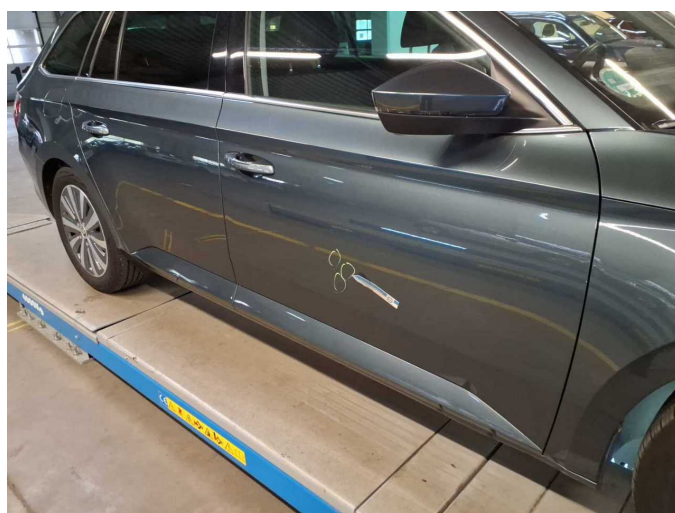
Damage 2: Door - front right side: Door - dent(s) - Smooth repair work
