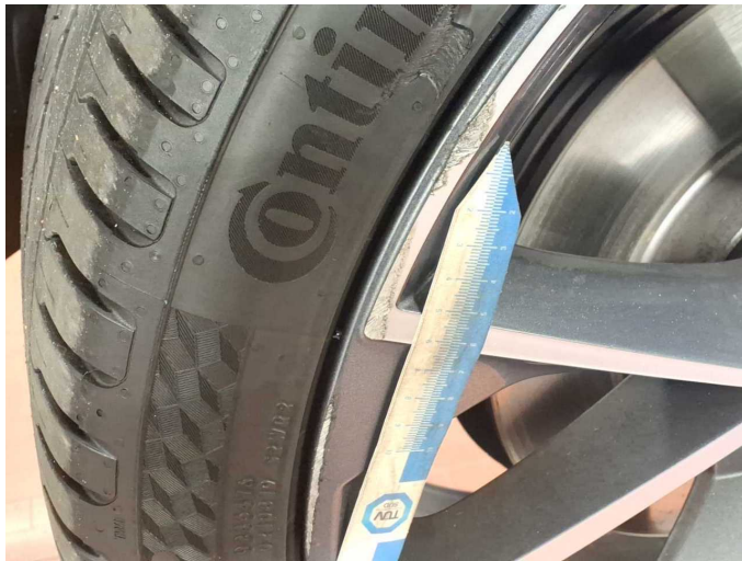
Damage 10: Wheel / tyres: Alloy rim - front right side - Scratched - Replace
