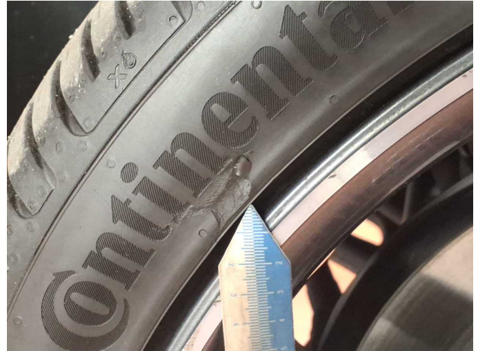
Damage 6: Wheel / tyres: Tyre - front right side - Damaged - Replace
