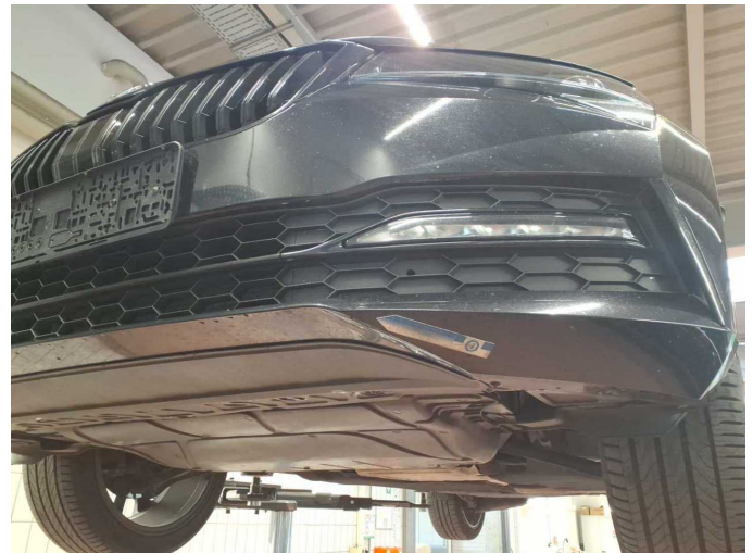
Damage 7: Front bumper: Front bumper (+ Steinschläge) - Scratched - Repair and paint
