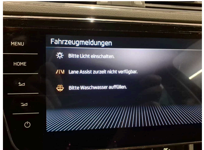
Damage 4: Electronic systems: Lane-keeping assistant - Electrical fault - Perform diagnosis
