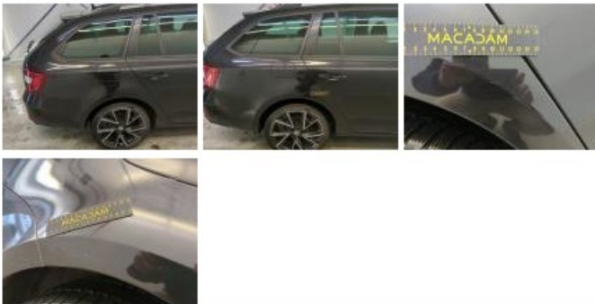
Door RR, Dent(s) and scratch(es), Repair and paint (complete)
