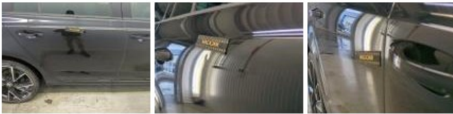
Outer door handle FR, Scratch(es), Repair and paint (complete)
