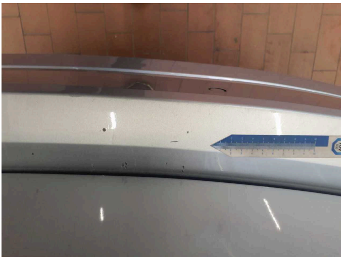
Damage 14: Rear bumper: Rear bumper - Scratched - Paint
