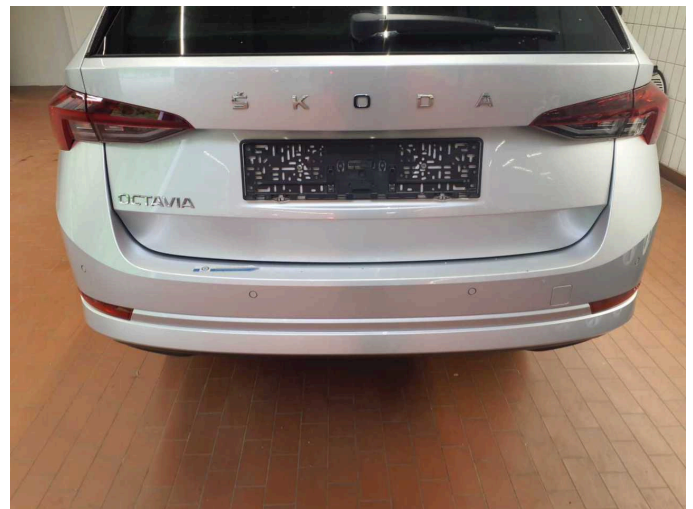
Damage 14: Rear bumper: Rear bumper - Scratched - Paint
