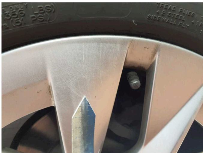
Damage 7: Wheel / tyres: Alloy rim - rear right side - Scratched - Smart repair
