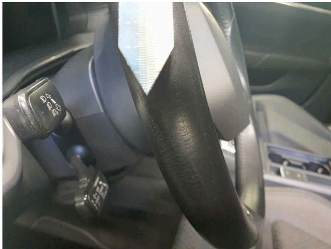
Damage 6: Steering system: Steering wheel - Scratch(es) - Smart repair
