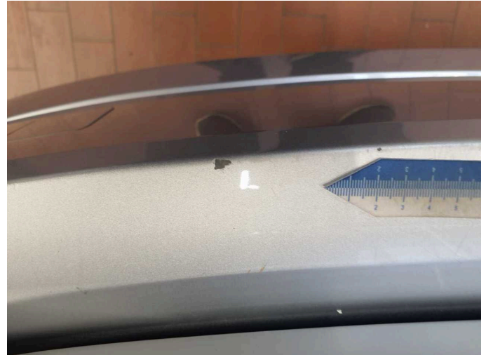
Damage 14: Rear bumper: Rear bumper - Scratched - Paint
