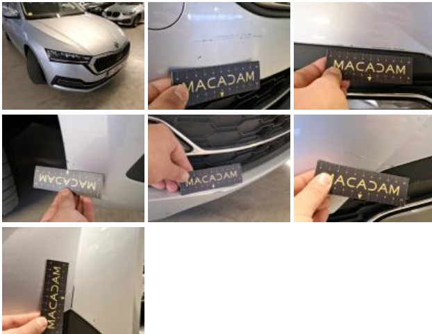
Bumper moulding F, Scratch(es), Replace
