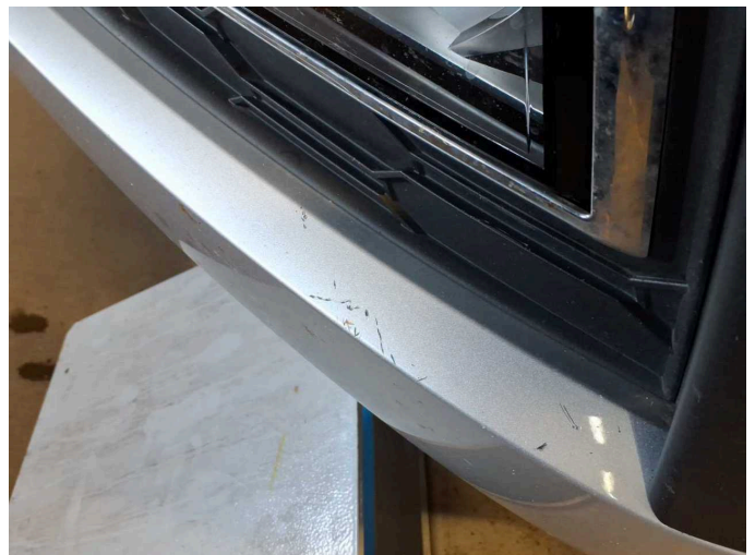
Damage 6: Front bumper: Front bumper - Scratched - Paint
