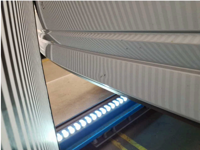
Damage 5: Rear bumper: Rear bumper (Leicht eingedrückt) - Scratched - Repair and paint
