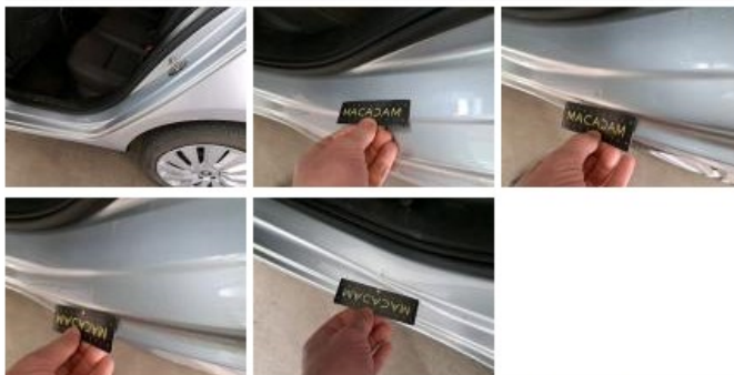
Door RL, Dent(s) and scratch(es), Spot repair
