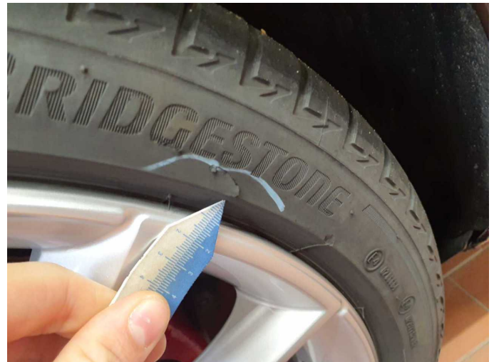
Damage 1: Wheel / tyres: Tyre - rear right side - Damaged - Replace
