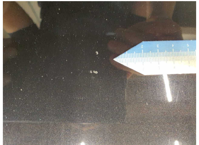
Damage 3: Bonnet: Bonnet - Stone chips - Paint
