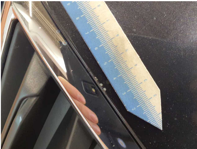
Damage 3: Bonnet: Bonnet - Stone chips - Paint
