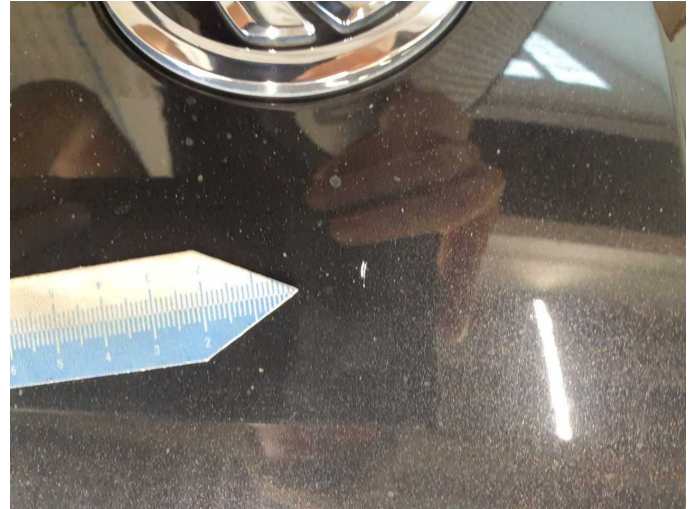
Damage 3: Bonnet: Bonnet - Stone chips - Paint
