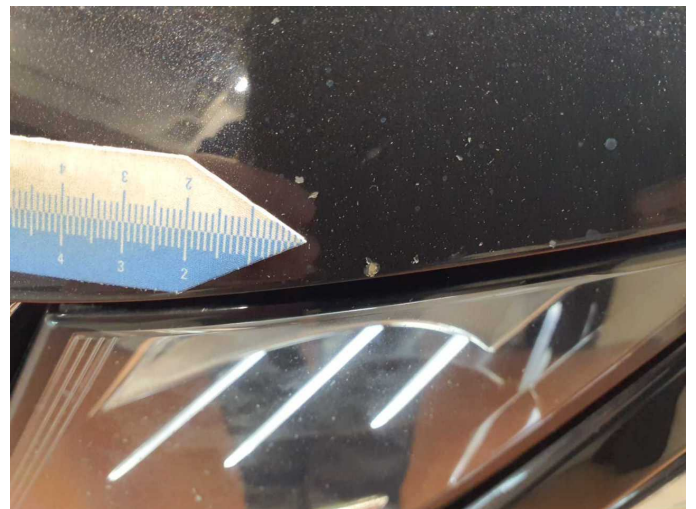
Damage 3: Bonnet: Bonnet - Stone chips - Paint
