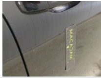
Door RR, Dent(s), Repair and paint (complete)
