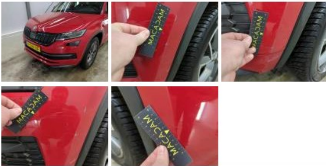
Bumper FM, Scratch(es), Repair and paint (complete)
