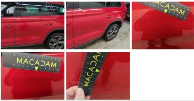
Door trim RL, Scratch(es), Replace and paint
