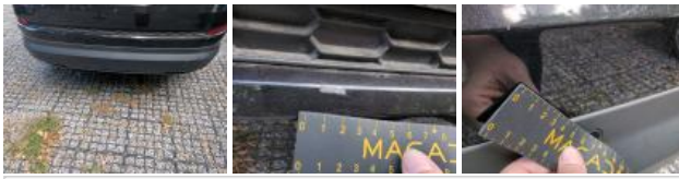
Wing trim RR, Dent(s), Replace
