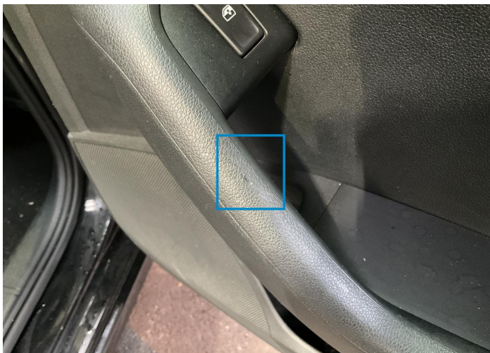
23. Interior door handle Back right Interior / Scratched -
