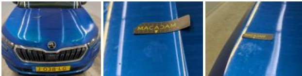
Wing RR, Dent(s), Repair and paint (complete)
