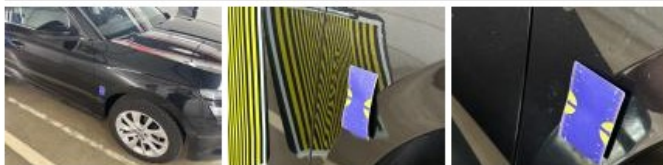
Outside rear-view mirror housing R, Scratch(es), Acceptable
