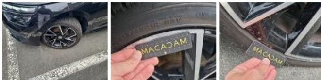
Step L, Dent(s), Acceptable
