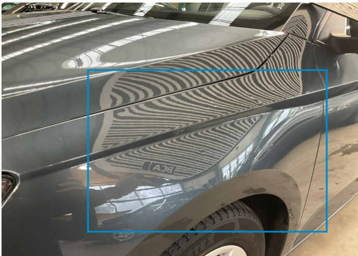
3. Fender / Front Left Bodywork / Dent / Hail Area -
