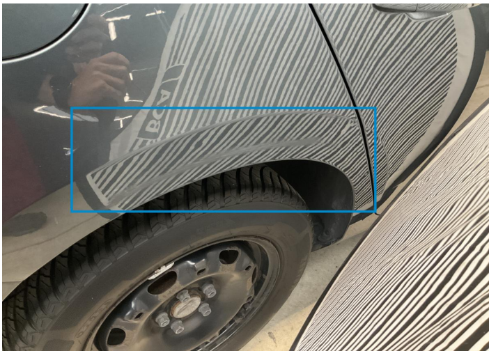
16. Fender / Back Right Bodywork / Dent / Dent -
