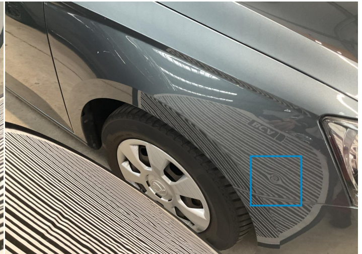
20. Fender / Front Right Bodywork / Dent / Dent -
