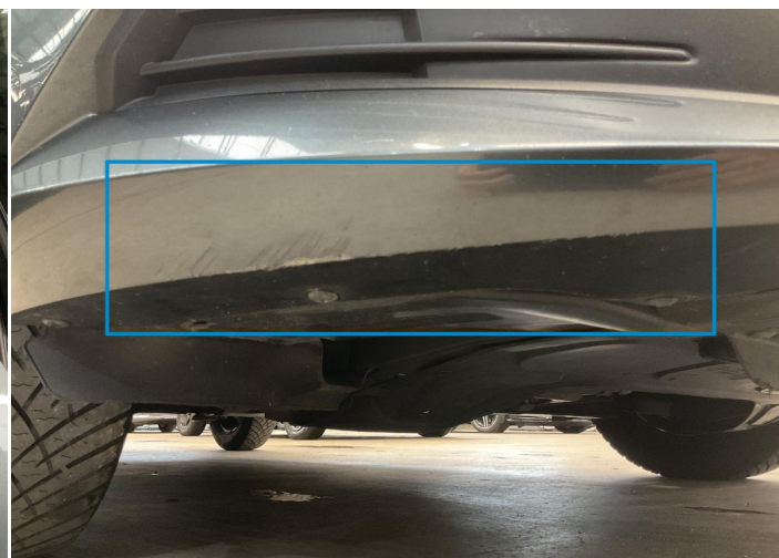
2. Bumper / Front Paint / Scratch / Scuff -
