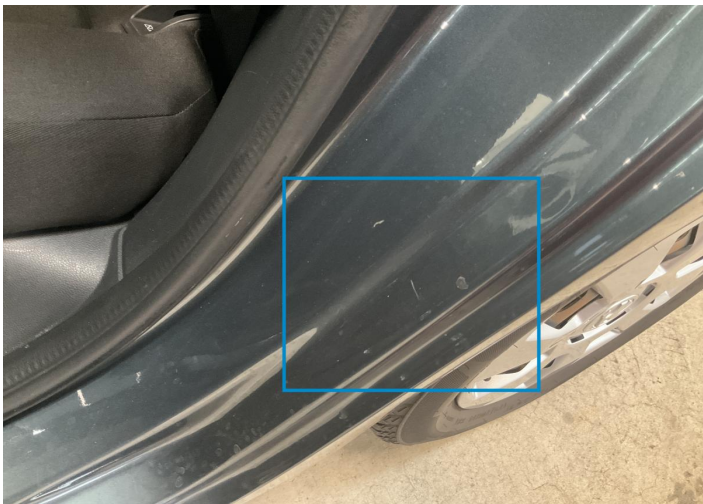
9. Pillar / Back Left Bodywork / Dent / Dent -
