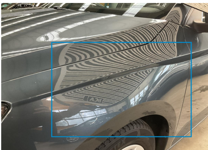
3. Fender / Front Left Bodywork / Dent / Hail Area -
