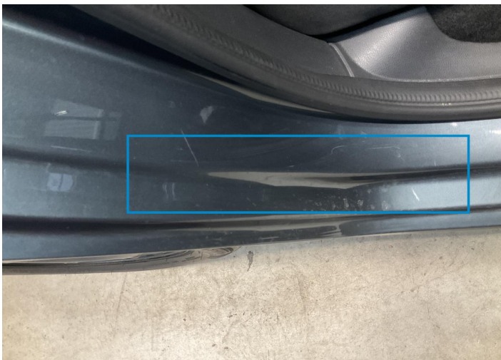
18. Pillar / Back Right Paint / Scratch / Scuff -
