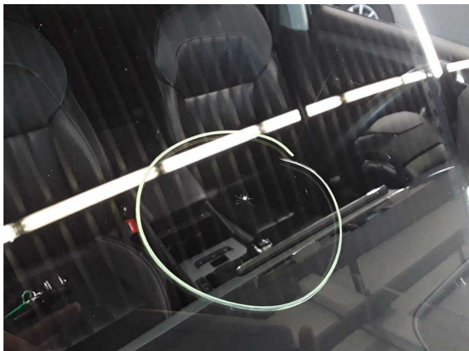
Damage 5: Vehicle glazing: Windscreen (Rissbildung) - Stone chips - repair according to calculation
