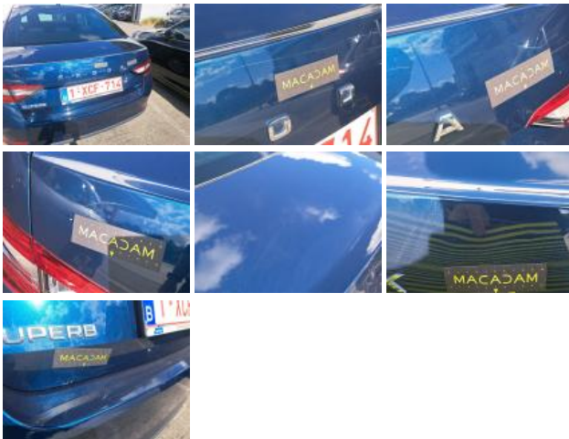
Bumper R, Scratch(es), Repair and paint (complete)
