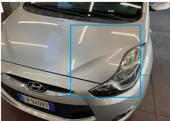
13. Hood Bodywork / Poor Previous Repair -
