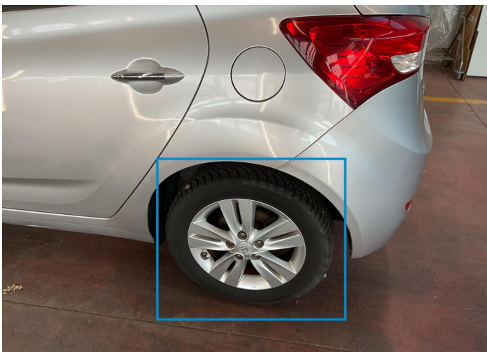
22. Rim / Back Left Out of Bodywork / Scratch -
