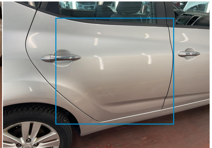
4. Door / Back Right Bodywork / Dent -
