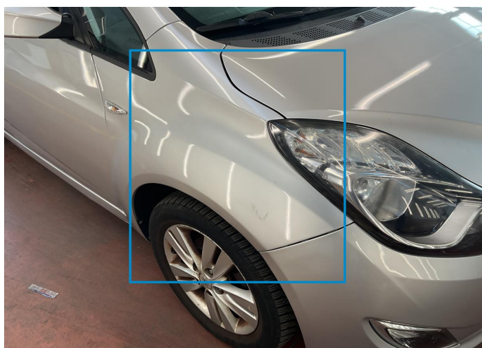
9. Fender / Front Right Bodywork / Poor Previous Repair -
