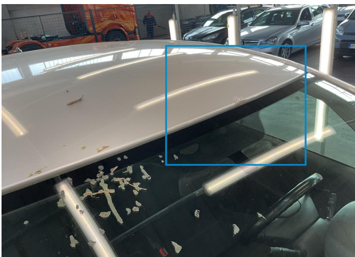
20. Roof Paint / Scratch / Line -
