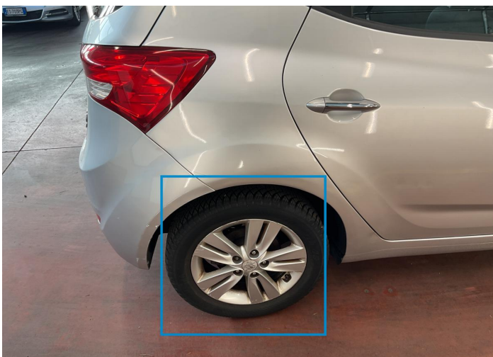
24. Rim / Back Right Out of Bodywork / Scratch -
