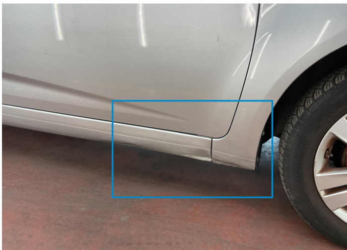
21. Rocker Panel / Center Right Bodywork / Dent -
