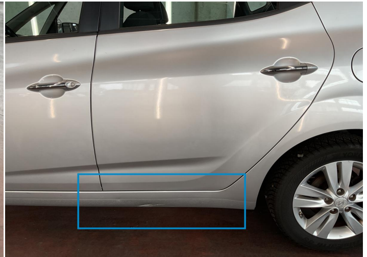
28. Rocker Panel / Center Left Bodywork / Dent -
