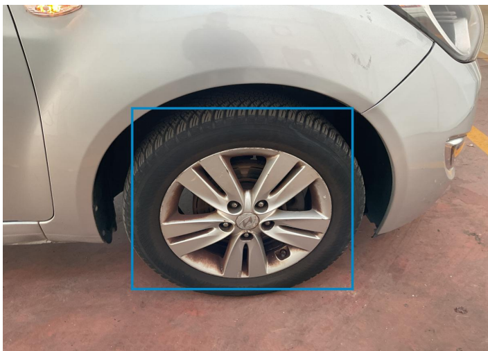
15. Rim / Front Right Out of Bodywork / Scratch -
