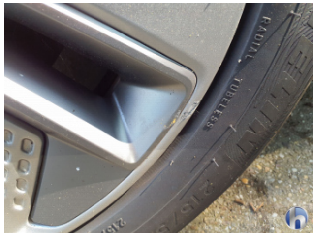
1. Rim front - left Deep scratch - Smart repair
