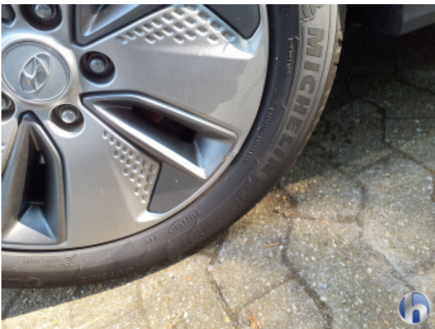
1. Rim front - left Deep scratch - Smart repair
