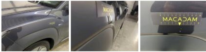
Outer door handle RL, Scratch(es), Repair and paint (complete)
