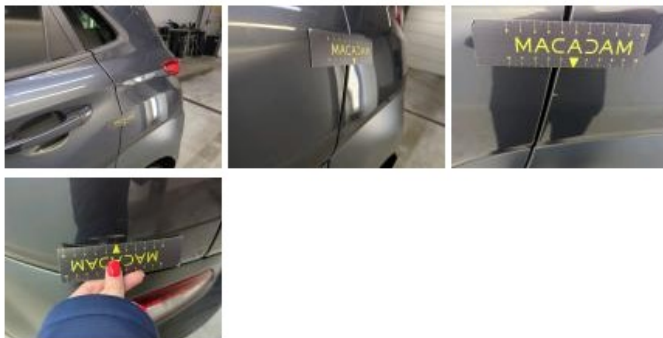
Bumper F, Scratch(es), Repair and paint (complete)
