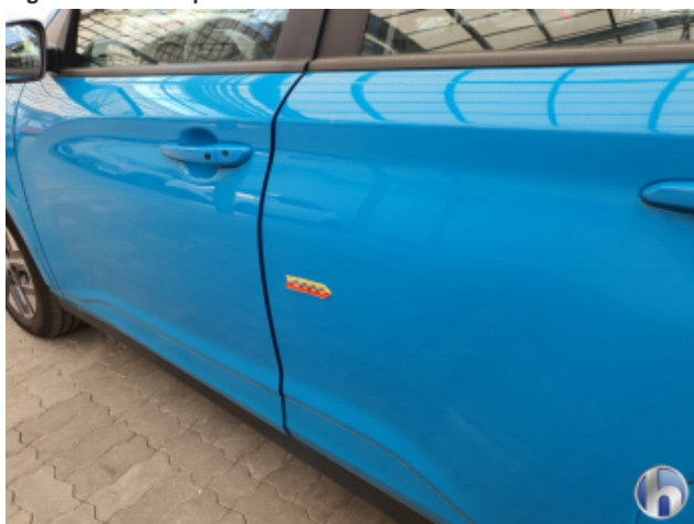
7. Rear door - left Surface scratch(es) - Condition/polish
