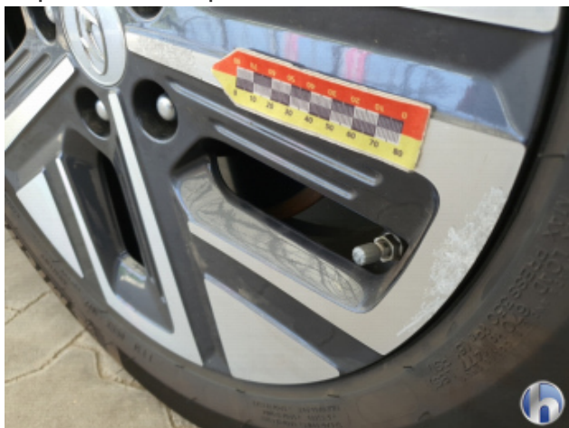
5. Rim front - right Deep scratch - Smart repair
