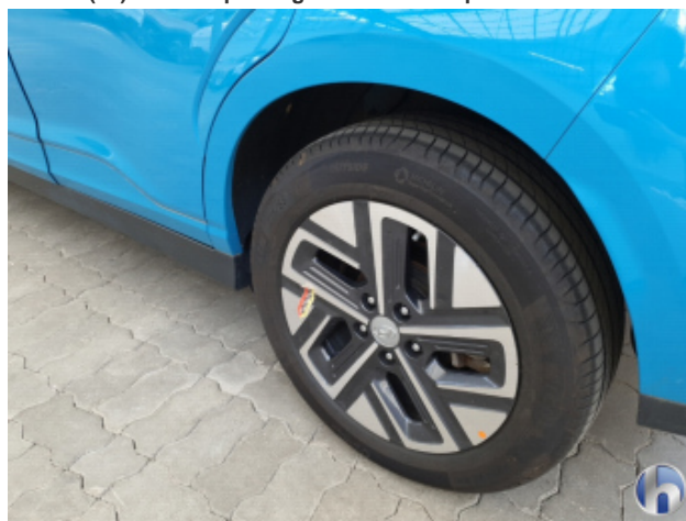
3. Rim rear - left Deep scratch - Smart repair
