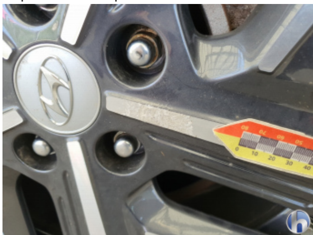
5. Rim front - right Deep scratch - Smart repair
