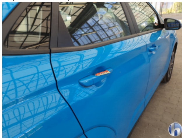
4. Outside Door Handle Rear - right Deep scratch - Smart repair
