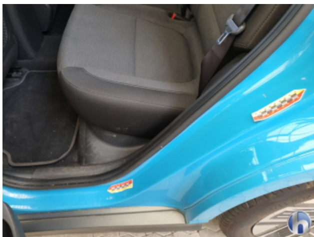
2. Türeinstieg Hinten - Links Scratch(es) down to priming coat - Smart repair
