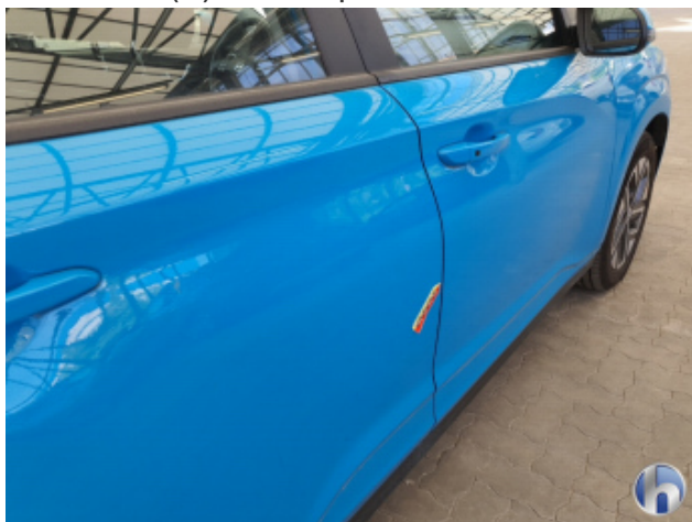
8. Rear Door - Right Surface scratch(es) - Condition/polish
