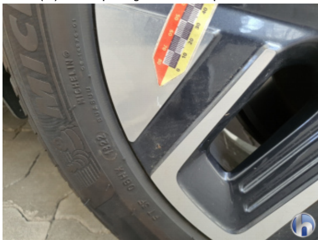
3. Rim rear - left Deep scratch - Smart repair
