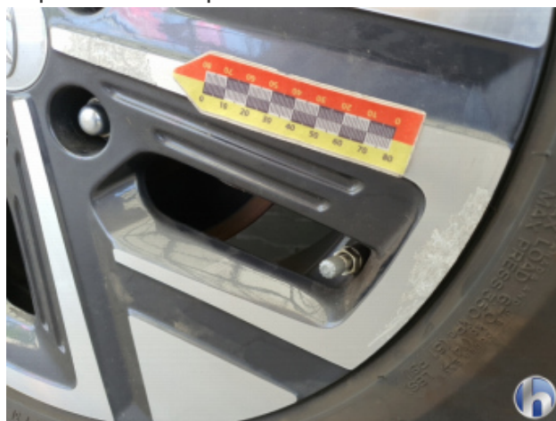
5. Rim front - right Deep scratch - Smart repair
