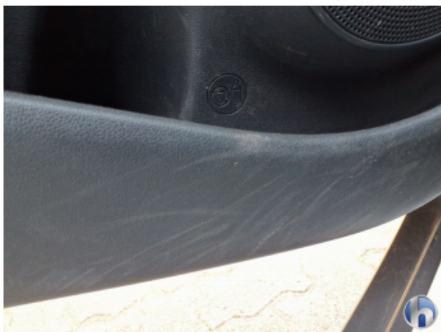
16. covering Wear and tear - Without repair
