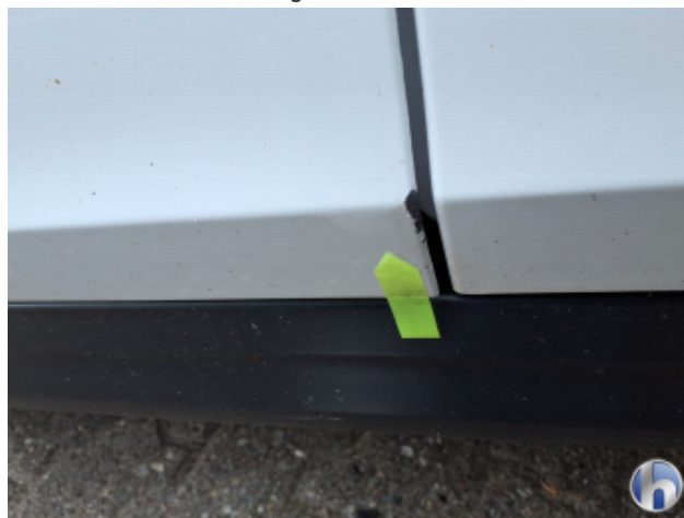
9. Front door - left Deep scratch - Smart repair
