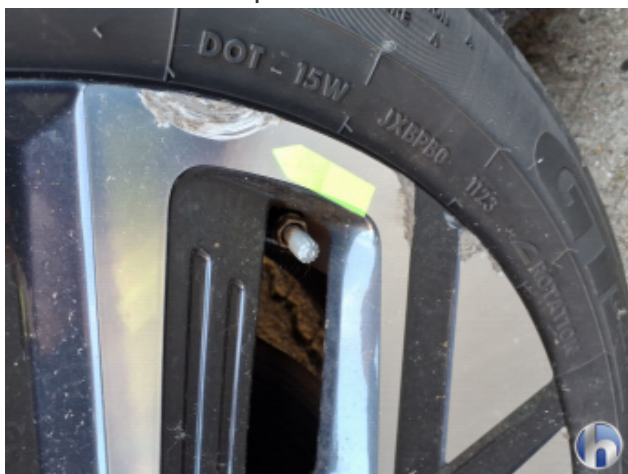
6. Rim front - left Damaged - Smart repair
