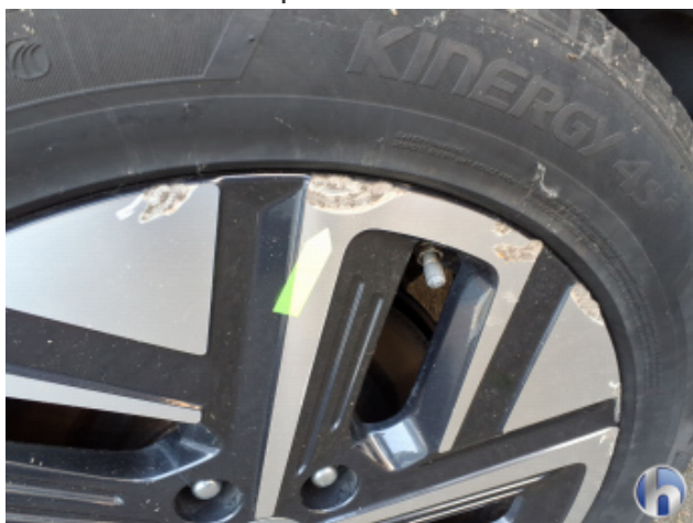
12. Rim rear - right Damaged - Smart repair
