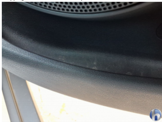
15. covering Wear and tear - Without repair
