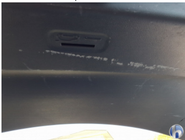
18. tailgate trim Damaged - Replace
