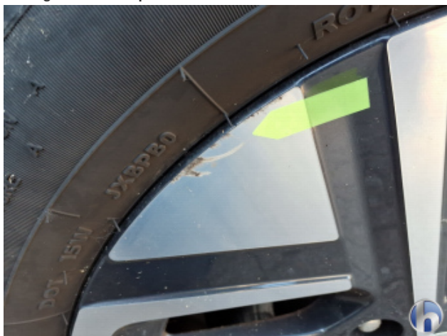
14. Rim front - right Damaged - Smart repair
