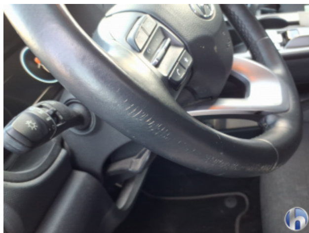
17. Steering wheel (leather) Deep scratch - Replace
