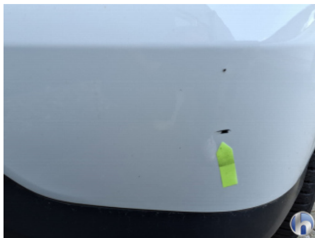
11. Rear Bumper Deep scratch - Smart repair
